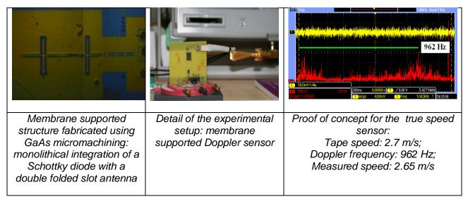
New design of the membrane supported structure (Electromagnetic modelling and optimization): the mask manufacturing, the characterization of the structures was performed using the IMT infrastructure. Manufacturing of the membrane supported antenna was performed in collaboration with FORTH Heraklion.
